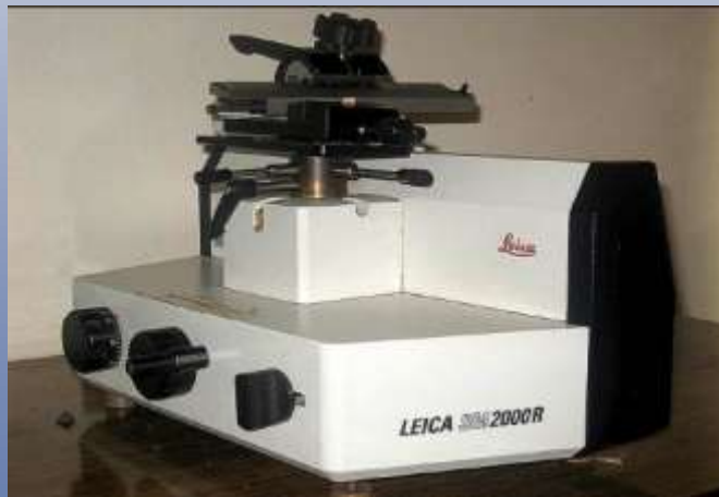
Sliding wood microtome (Leica SM 2000 R) used for wood sectioning
