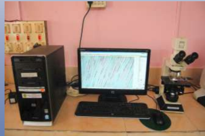
Image Analyser (Labomed Digi-2) used for anatomical quantification
