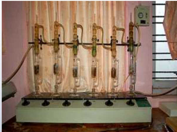
Determination of heartwood extractive content using Soxhlet apparatus
