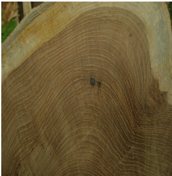
Fig 1. End- grain pattern showing distinct sap wood and heart wood; distinct growth rings and coarse texture of wood.
